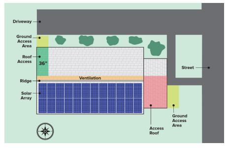
Again using the same example, with the adjoining roof within 24 inches of the array roof. Applying exception #3 you would only need a single access point and pathway on the main roof, as there is secondary access via an adjoining roof within 24 inches. This still allows two directions of egress, and does not share a common truss of rafter.
