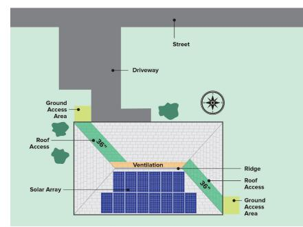
R324.7.5 Typical Hip Roof, showing alternate venting location and clear access pathway not less than 36 inches wide (914 mm) extending from the roof access point to the ridge or peak. Access and egress is from opposite sides and does not rely on the same roof truss or rafter and clear ground access.
