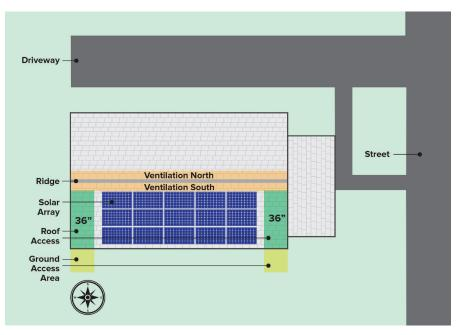
Using the original example, but now shown without any exceptions where vertical ventilation techniques will be employed would result in a smaller array. It's important to understand the exceptions and when they apply in order to maximize the available roof space.
