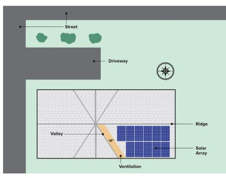
This image shows the 18 inch clear space from the valley to the array. The access and egress paths are not shown for clarity, nor is the venting location. There is street access to the front, and possible alternate venting on the opposite roof slope.
