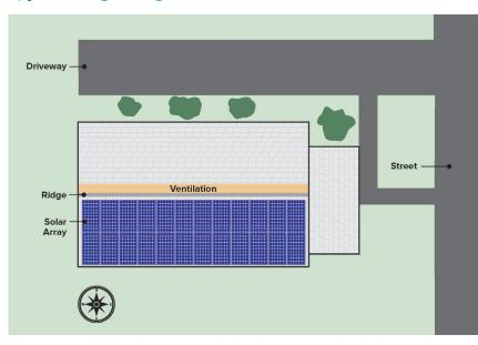
If ventilation is required it may be possible to propose an alternate ventilation location on roof slope opposite the array or the side wall of an attic space. Alternate locations should be coordinated and approved by the AHJ.
