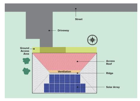
Using the same HIP roof example, exception #2 would apply for all residential structures where an access roof fronts a street, driveway, or other area readily accessible to emergency responders. "**R324.7.6 Roofs with valleys.** Panels and modules shall not be located less than 18 inches (457 mm) from a valley. Exception: Roofs with slopes of 2 units vertical in 12 units horizontal (16.6 percent) and less."
